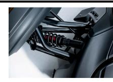
**FULL KYB HPG SHOCKS** Front and rear KYB HPG shocks with rear remote adjuster for different riding experiences.
